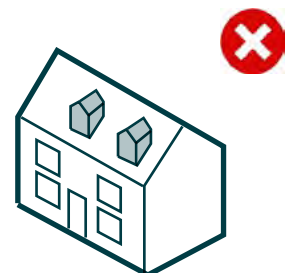
Loft conversion incorporating gable dormers which are out of scale.
