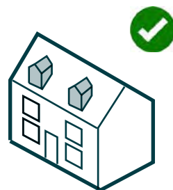
Loft conversion incorporating gable dormers.
