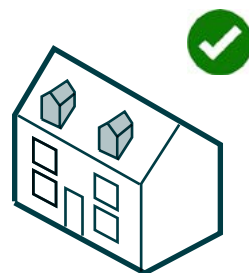
Loft conversion incorporating gable dormers.
