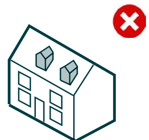
Loft conversion incorporating gable dormers which are misaligned.
