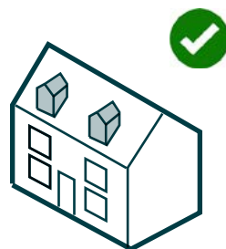
Loft conversion incorporating gable dormers.
